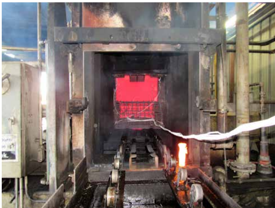
A temperature uniformity survey on an internal quench furnace.
